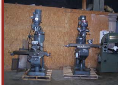
Partial view of Vertical Mills
