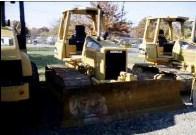
OROPS Blade/Width: PAT 116" Track Length: 112" Track Shoes: 25"
