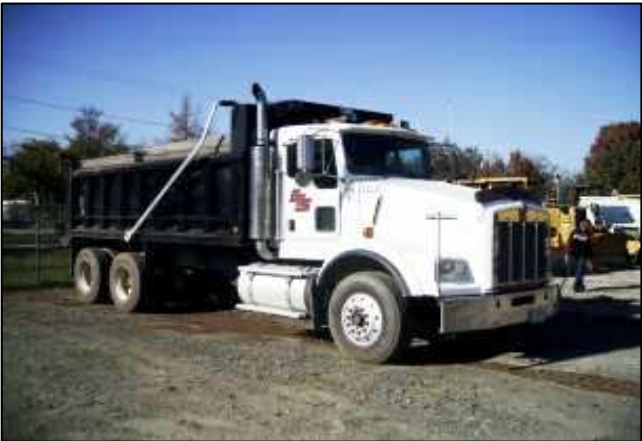
WB: 226" Bed Length: 17' Bed Width: 8' 16yd Tandem Axle
